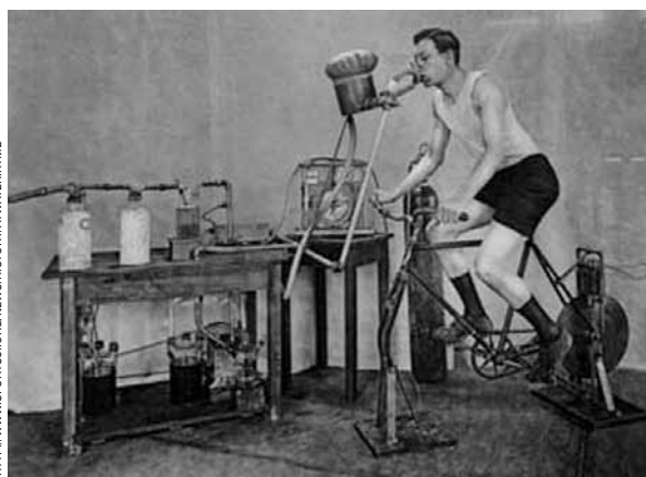
This exercise machine, called an ergometer, was used in the laboratory of Wilbur Olin Atwater to measure the amount of calories released by exercising.
