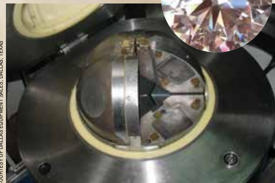
A high-pressure high-temperature diamond crystal growth chamber is used to make synthetic diamonds, such as the one shown above.
