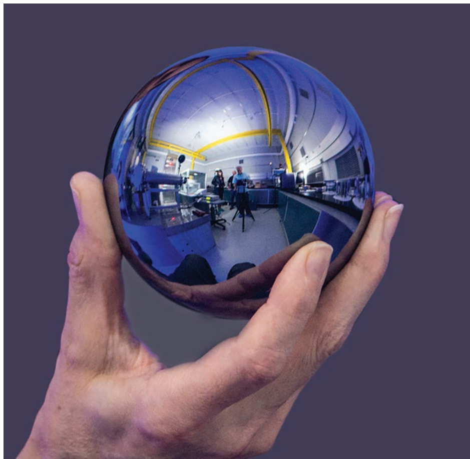
⤴ A silicon sphere similar to this one was used to redefine the Avogadro constant.
