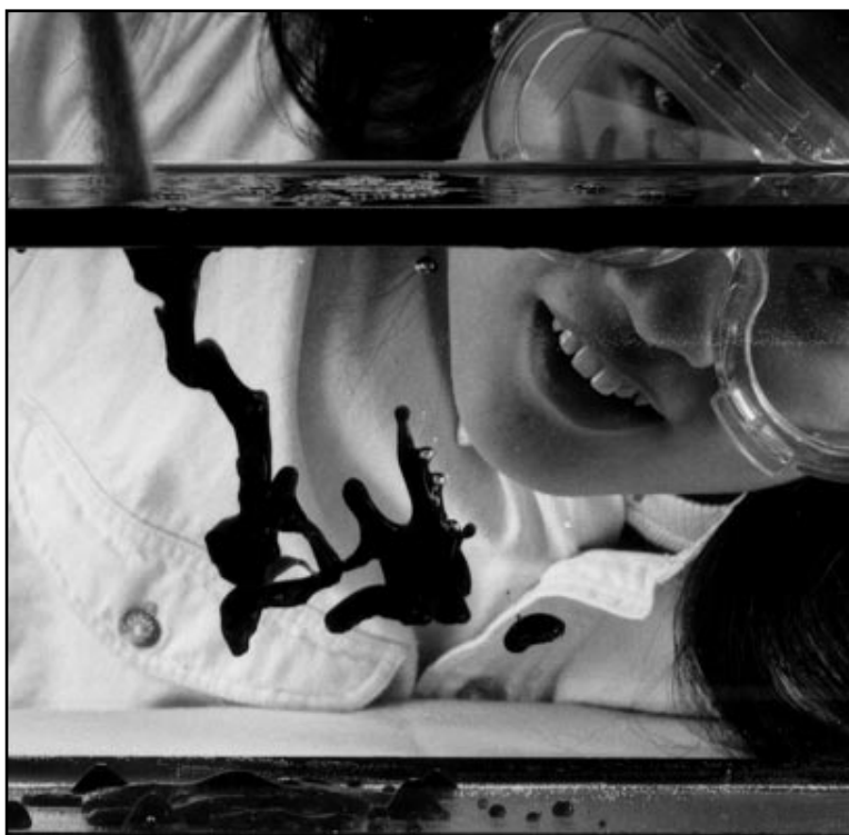
This experiment begins with a layer of motor oil floating on water (top photo). When Magic Sand is added (bottom photo), it sinks and carries a glob of oil with it to the bottom.
